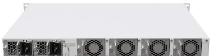
There are **2x QSFP28** cages for blazing-fast 100 Gigabit connectivity, **12x SFP28** cages for 25 Gigabit networking, and a **Gigabit Ethernet** port. The device comes with **16 GB of RAM**, decent **NAND** storage, and **two M.2 SATA slots** for additional storage. There are four hot-swappable fans, as well as dual-redundant hot-swap power supplies. And these PSUs might look familiar if you have used our CCR1072 before: you can keep using your previous hot-swap power supplies and SFP modules.
