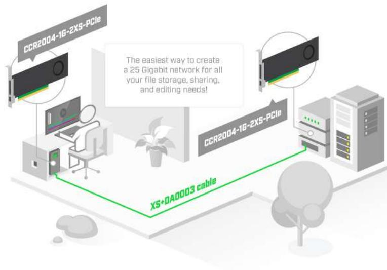
This form-factor does come with certain limitations that you should keep in mind. The CCR NIC card needs some time to boot up compared to ASIC-based setups. If the host system is up before the CCR card, it will not appear among the available devices. You should add a PCIe device initialization delay after power-up in the BIOS. Or you will need to re-initialize the PCIe devices from the HOST system.
