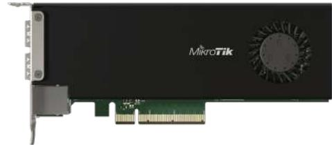
By default, the PCIe interface will show up as four virtual Ethernet interfaces. Two interfaces in passthrough mode to the 25G SFP28 cages. Remaining two virtual Ethernet-PCIe interfaces are bridged with the Gigabit Ethernet port for management access. The user can configure all interfaces and settings freely since we are running fully functional RouterOS here.
